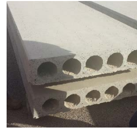
Hollow Core Designs Offer a Light Weight Alternative (Alqattan, 2013)
